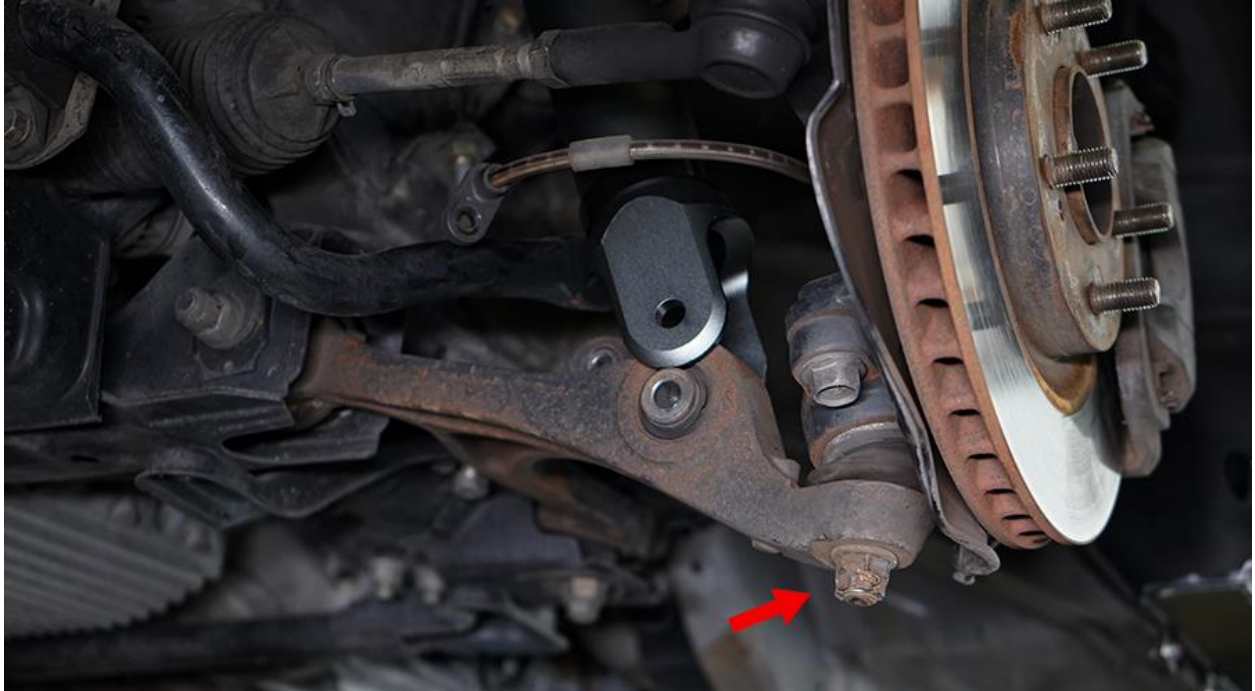
Insert ball joint back into lower control arm, tighten down and make sure to install a new cotter pin.
