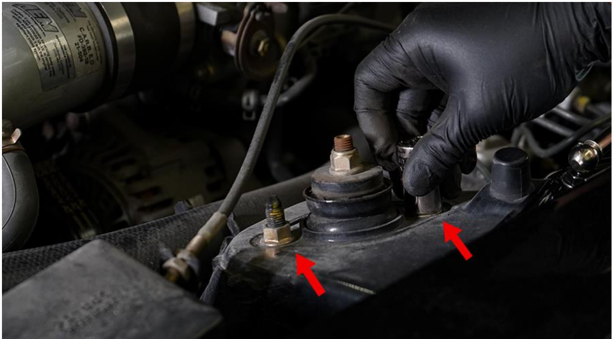
Remove both top mount nuts.
