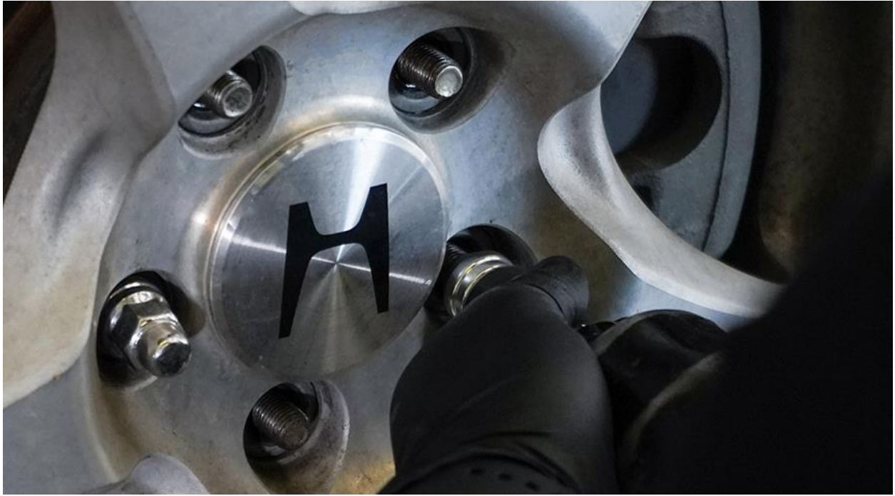
Remove Lug nuts and wheel
