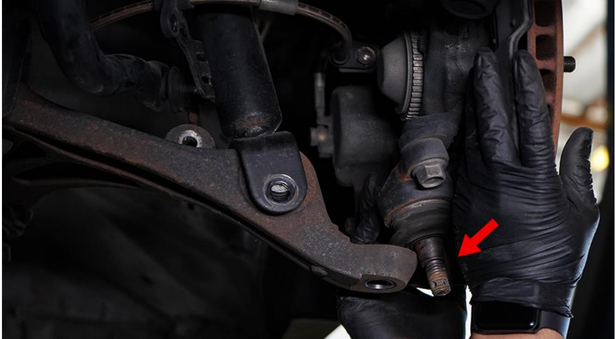
Remove castle nut and lift out ball joint out of lower control arm.
